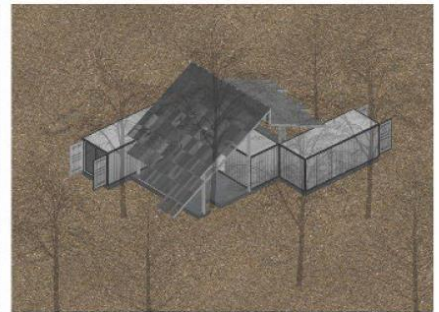
6. roof layer with solid and transparent material blending with the surrounding foliage shadow
