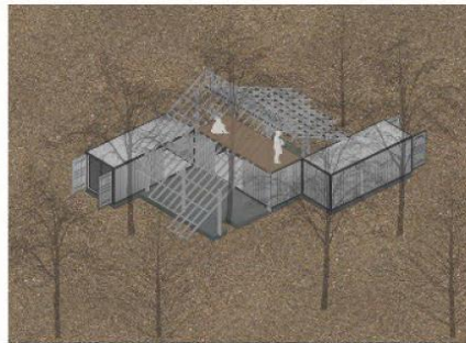
5. steel structure install + additional space over common room container unit
